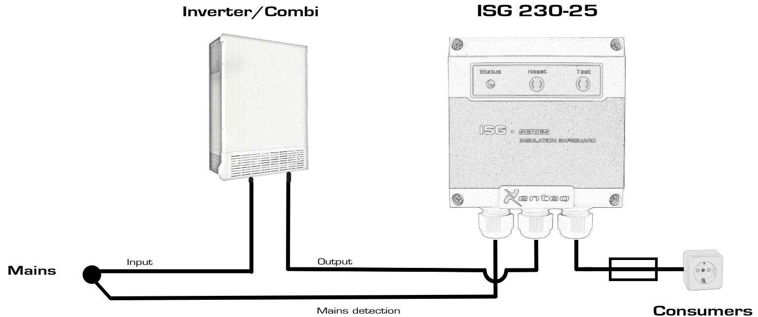
**Important:** There must be no voltage on the mains voltage detection cable when the inverter is in operation! This is relevant for devices with a priority switch where the inverter has priority over the mains voltage.
