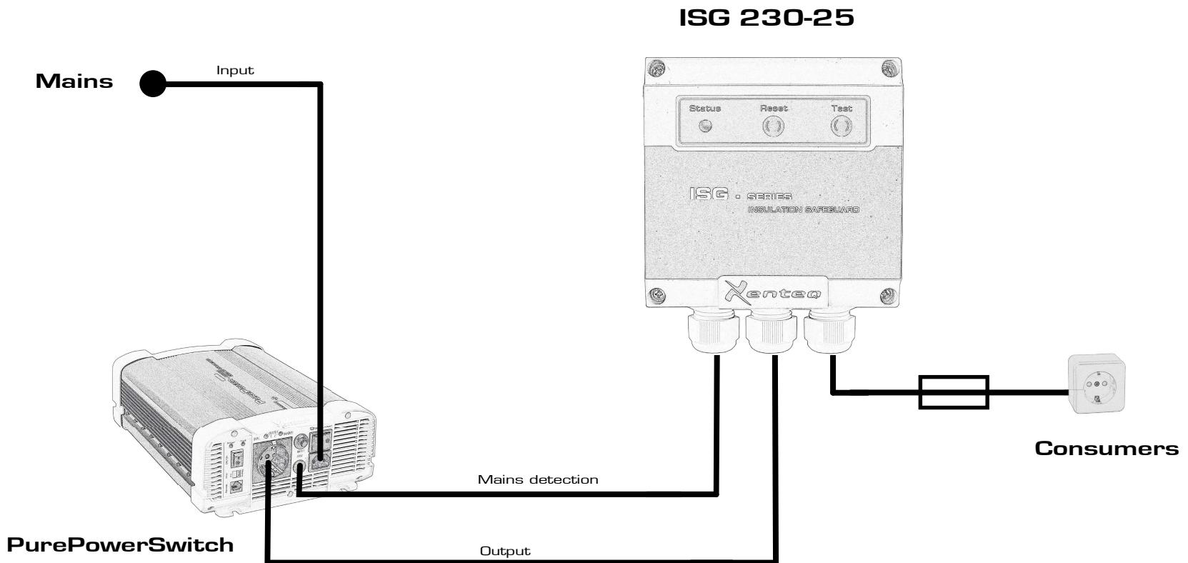
**Important:** Always connect the mains voltage detection (sense wire) connection of the ISG insulation safeguard to the 'MD' connector of the PurePowerSwitch. Use the cable supplied with the PurePowerSwitch for this.
